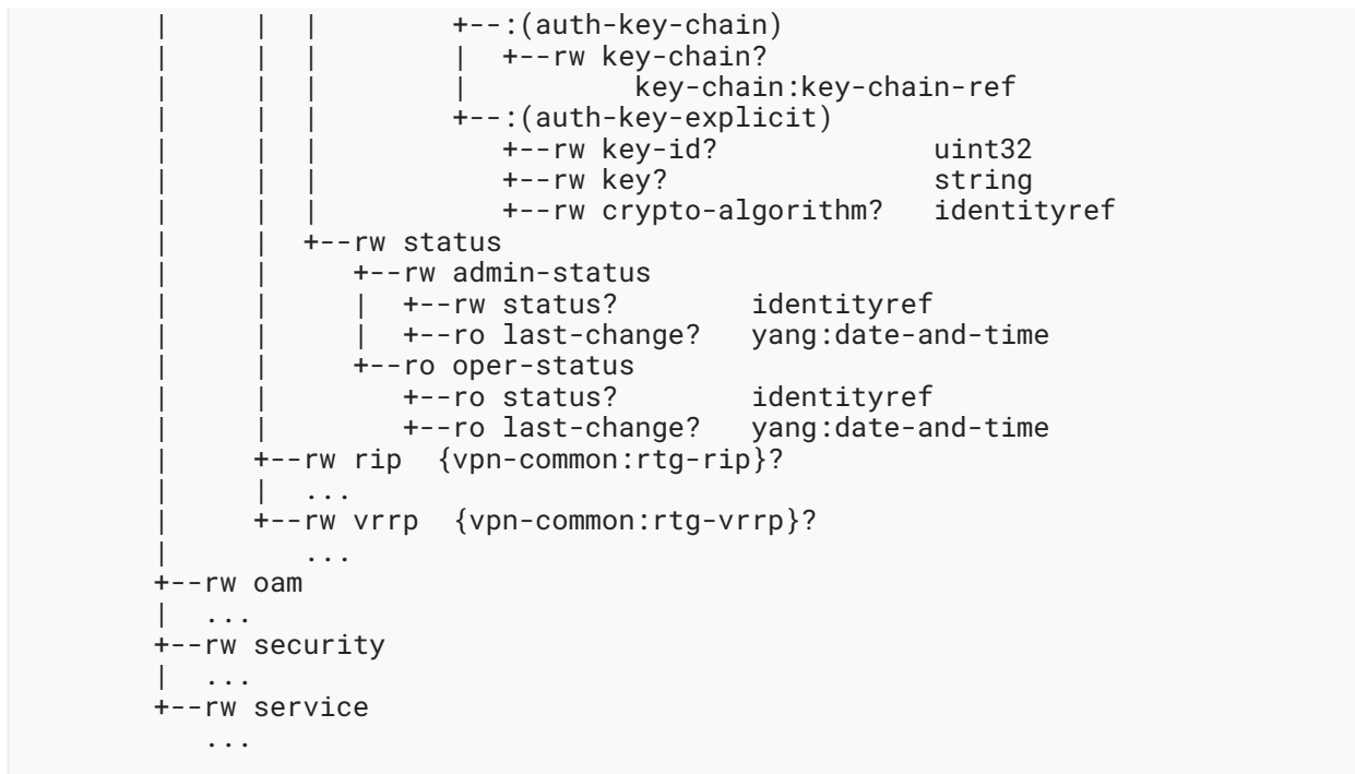
Figure 15: IS-IS Routing Tree Structure
