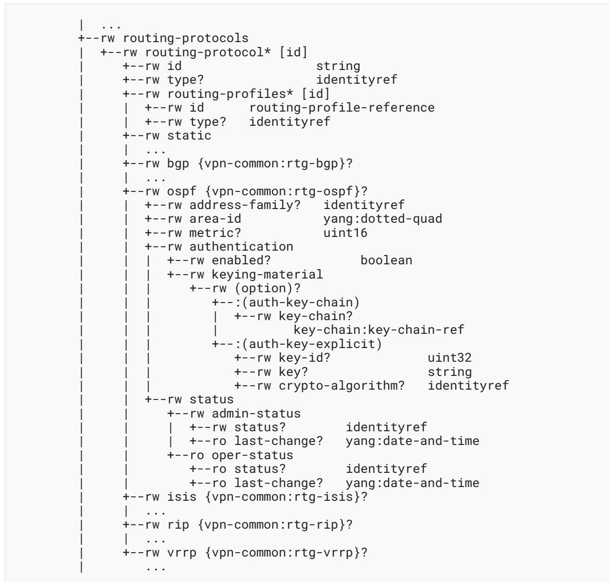
Figure 17: OSPF Tree Structure
