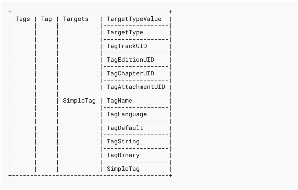
Figure 10: Representation of a Tags Element and Three Levels of Its Children Elements
